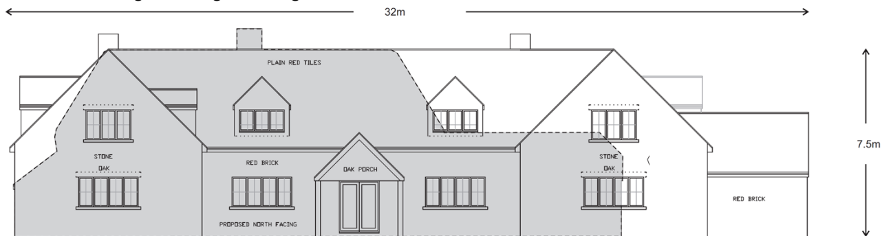
Proposed front elevation with the size of the previous cottage superimposed in grey for comparison
